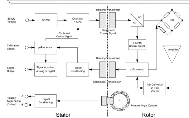
Block diagram for serial signal transmission
