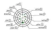
View: socket on soldering side
