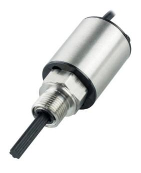
A choice of output types is available: analog voltage in two spans, 0.5-4.5V or 0.2-4.8V; 4-20mA current loop; or one of three PWM frequencies. Each of the output types can have its full span set to correspond to the selected measurement range, while the polarity of the output is also configurable. The sensor and associated electronics are also shielded against electromagnetic disturbances.
