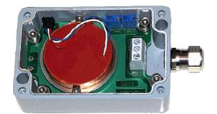
Sensor box containing one sensor and one signal condtioner with 4...20mA, 2-wire output
