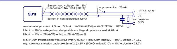
Since the SB1I supply voltage feeds off the current loop (the SB1I requires 3mA at most), a voltage of 10V across the SB1I terminals must be guaranteed to ensure correct functionality even for the maximum loop current of 24mA (maximum voltage drop across transmission line and load resistance).
