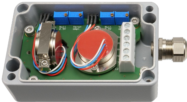
Sensorbox containing two sensors and two signal conditioners with 0.5 to 4.5 Volt signal outputs
