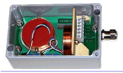
Sensor box containing two NG inclinometers and two signal conditioners with 0...5V outputs and extensive temperature drift compensation
