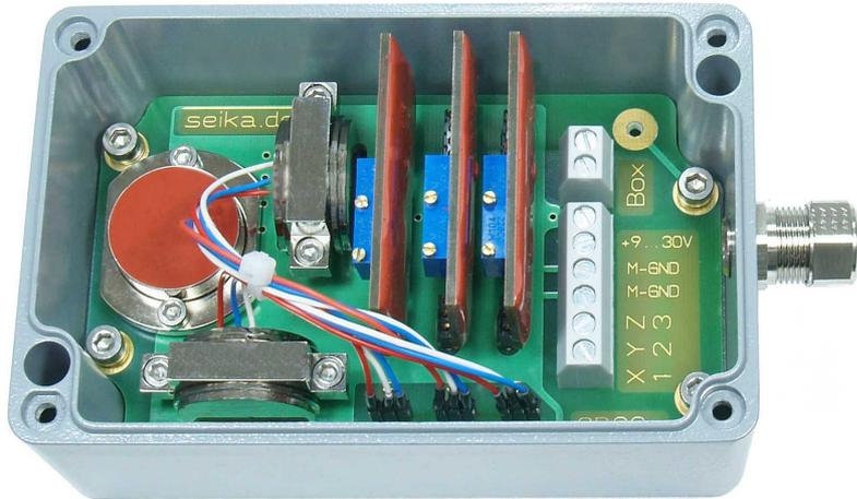
**Sensor box containing three SEIKA sensors and three signal conditioners with 0...5V or +/-4V output.**
