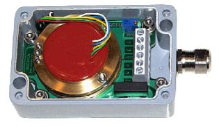
Sensor box containing one highly sensitive servo inclinometer and one signal conditioner with ±5V output
