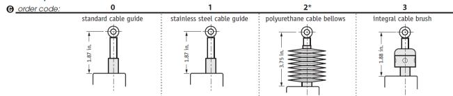
\*important! – bellows limits measuring cable travel to 25 inches, contact factory before ordering.
