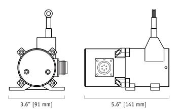
The PT8232 delivers position feedback via RS232 serial communication to your data acquisition or controller system. The PT8232 sends a raw 16-bit count from 0000H to FFFFH. Additionally this device can be set to continuously send data or send data only when polled.
