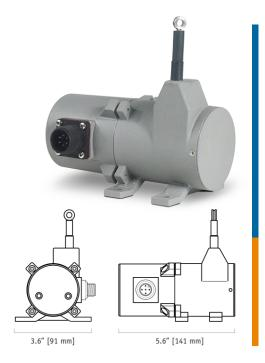
The PT8DN, using a high cycle plastic-hybrid potentiometer, communicates via DeviceNET protocol with programmable controllers in factories and harsh environments requiring linear position measurements in ranges up to 60".
