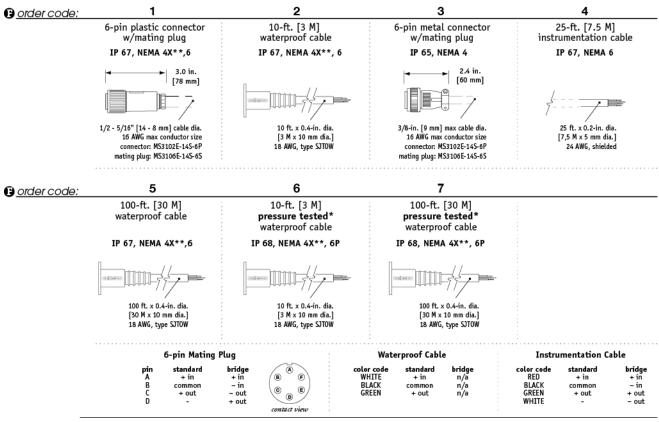
Notes: \*-Test pressure: 100 feet [30 meters] H2O (40 PSID); Test Medium: Air; Duration: 2 hours. \*\*-NEMA 4X applies to stainless steel enclosure only.
