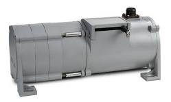
The PT9232 delivers position feedback via RS232 serial communication to your data acquisition or controller system. The PT9232 sends a raw 16-bit count from 0000H to FFFFH. Additionally this device can be set to continuously send data or send data only when polled.
