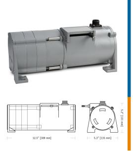
The PT9301 is a combination position and velocity transducer for demanding long-range applications requiring a linear position measurements in ranges up to 1700". A precision plastic-hybrid potentiometer provides accurate position feedback while a self-generating DC tachometer provides a velocity signal that is proportional to the speed of the traveling stainless-steel measuring cable.
