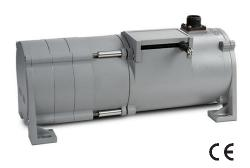
The PT9510 can operate from an unregulated 14.5 to 40 VDC power supply while providing a regulated output signal over its full extended range of up to 1700". It provides a 0 - 10 VDC position feedback signal proportional to the linear movement of its stainless steel measuring cable.
