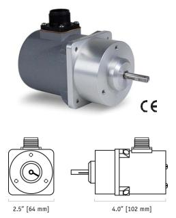
Celesco's model RT8101 provides a voltage feedback signal for rotational position. The sensing element of this device is a precision plastic-hybrid potentiometer which provides superb linearity and resolution.
