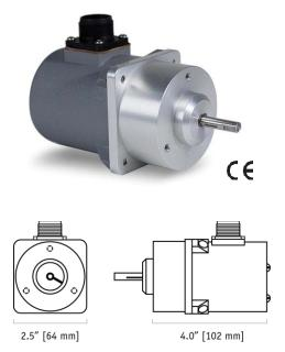
The RT8510 can operate from an unregulated 14.5 to 40 VDC power supply while providing a regulated output signal over its full range from 1/8 of a turn up to 200 turns. It provides a 0 -10 VDC position feedback signal proportional to the rotational position of the shaft
