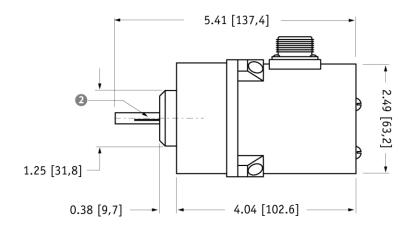
mounting holes: for .25 in. shaft option, mounting holes are threaded #10-32 x 0.375 deep 120° apart on a 2.00 inch dia. BC
