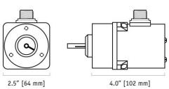
Our model RT8DN communicates rotational position feedback via DeviceNET® to your programmable controller. The heart of this sensor is a precision plastic-hybrid position potentiometer which provides an "absolute" position and does not ever have to be reset to a "home" position after a power loss or planned shutdown.
