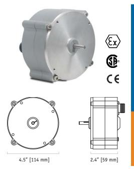
The RT9420 provides rotational position feedback via 4...20 mA current loop signal. This device combines the superb linearity and resolution of a plastic-hybrid potentiometer and the durability of Celesco's 4...20mA circuit to provide an accurate and reliable electrical signal. Additionally the zero and span settings are adjustable through access holes in the housing.
