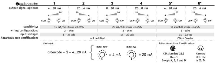
\*IMPORTANT: intrinsically safe when powered from a CSA certified zener barrier rated 28 VDC max, 110 mA max per installation drawing#677984
