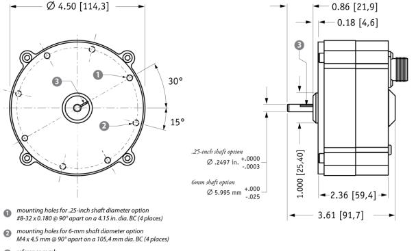
eference mark full counter-clockwise position - align mark on shaft to mark on face for start of measurement range
