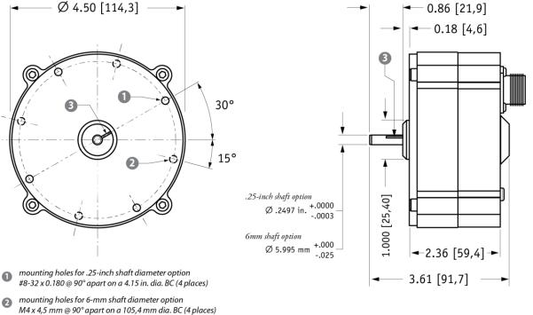
reference mark full counter-clockwise position - align mark on shaft to mark on face for start of measurement range
